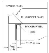
3/4 (19)typical Panel assembly rear view.
