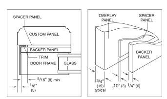
Panel assembly cross section. Panel assembly rear view.
