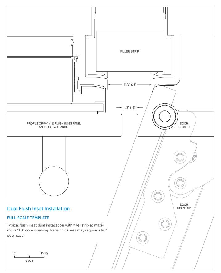
Dual flush inset installation (top view)
