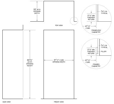
NOTE: 3<sup>1</sup>/2\* (89) finished returns will be visible and should be finished to match cabinetry.
