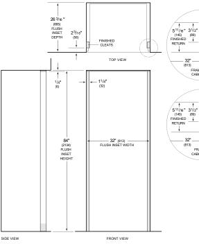
$NOTE: 3^{1}\!/z^*(89) \text{ finished returns and shaded areas will be visible and should be finished to match cabinetry Shaded line represents profile of unit <math display="inline">\textbf{hr} i k / t^*(19) \text{ panel}.$
