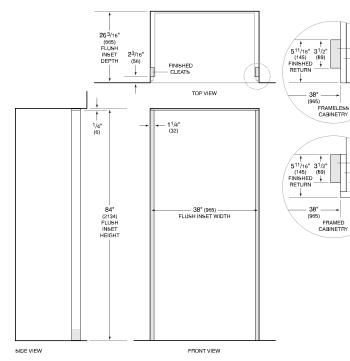
NOTE:  $3^{1}/2^{n}$  (89) finished returns and shaded areas will be visible and should be finished to match cabinetry. Shaded line represents profile of unit with  $3^{1}/4^{n}$  (19) panel.
