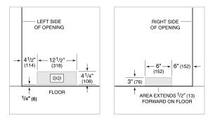
NOTE: The electrical outlet must be positioned with the grounding prong to the right of the thinner blades.
