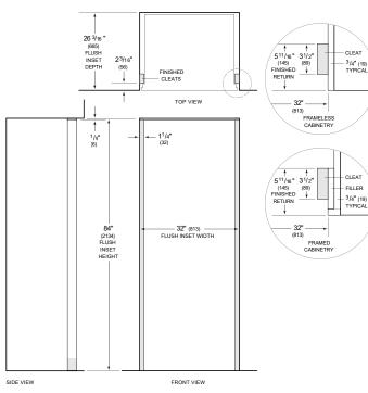
NOTE: 31/2" (89) finished returns and shaded areas will be visible and should be finished to match cabinetry Shaded line represents profile of unit wi{/4" (19) panel.
