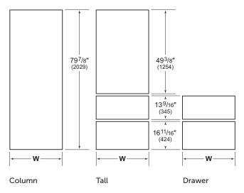
Typical panel dimensions are based on an 84" (2134) finished height for column and tall models and  $34^{1/2}$ " (876) for drawer models, with a 4" (102) toe kick and  $\frac{1}{8}$ " (3) reveals. Panel dimensions must be adjusted accordingly for all other installations. Refer to the illustration for panel height and the chart below for panel width.
