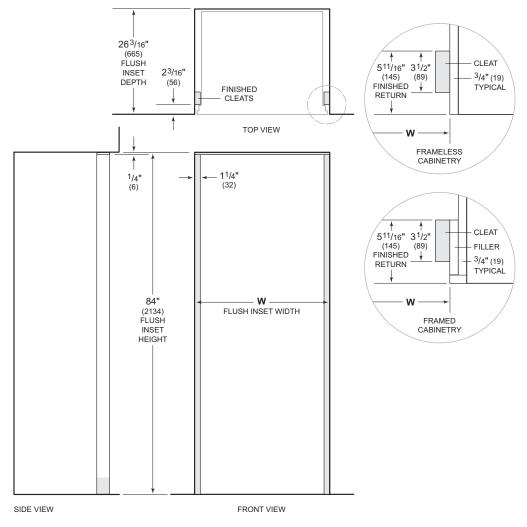
NOTE:  $3^{1/2}$ " (89) finished returns and shaded areas will be visible and should be finished to match cabinetry. Shaded line represents profile of unit with 3/4" (19) panel.
