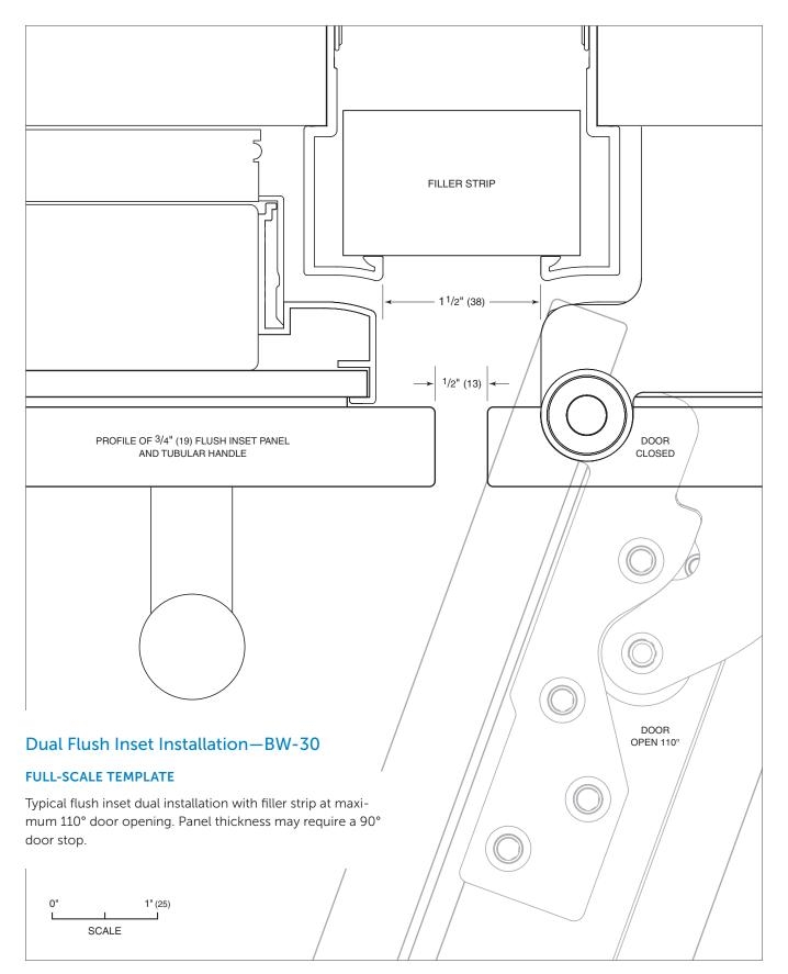
Dual flush inset installation (top view)
