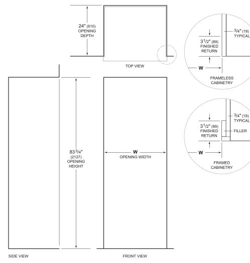
NOTE:  $3^{1/2^{\prime\prime}}$  (89) finished returns will be visible and should be finished to match cabinetry. Shaded line represents profile of unit.
