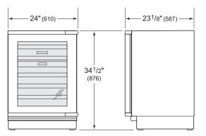
**IMPORTANT NOTE:** Overall dimensions do not include panels or handles. Dimensions will vary with panel thickness.
