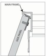
5 Rotate the back of the panel toward the unit, then shift the panel downward so the bracket hooks engage the side panel.
