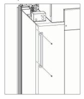
3 Install the base cover on the base support assembly.
