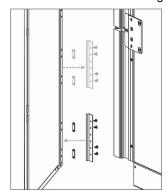
Install the upper and lower rear brackets with the provided screws. Verify the bracket hooks face upward.
