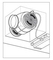
4 Install the mesh filters and rotate the bottom cover upward and into position.
