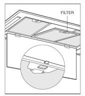
3 Place the recirculating filters on both sides of the blower and rotate the filters counter-clockwise to secure.
