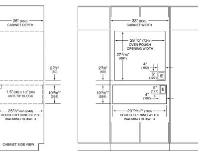
NOTE: Dimensions in parentheses are in millimeters \*Dimension may vary by ± 1/8" (3 mm).
