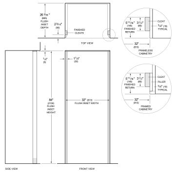
NOTE: 31/2" (89) finished returns and shaded areas will be visible and should be finished to match cabinetry Shaded line represents profile of unit **b**it/8/1" (19) panel.
