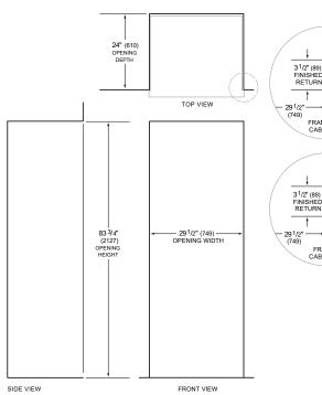
NOTE: 3<sup>1</sup>/2" (89) finished returns will be visible and should be finished to match cabinetry Shaded line represents profile of unit.
