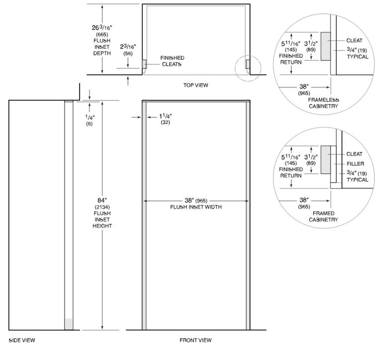
**NOTE:** 3/16" (89) finished returns and shaded areas will be visible and should be finished to match cabinetry. Shaded line represents profile of unit with 3/4" (19) panel.
