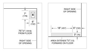
PANEL SPECIFICATIONS For complete panels specifications including width/height, weight requirements, thickness requirements and offset details visit subzerowolf.com/builtinconfigurator.
