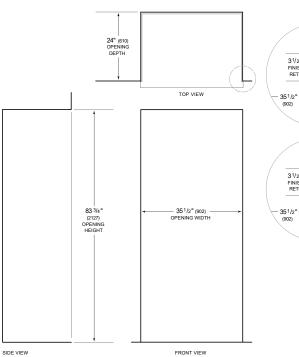
NOTE: 3<sup>1/2\*</sup> (89) finished returns will be visible and should be finished to match cabinetry Shaded line represents profile of unit.
