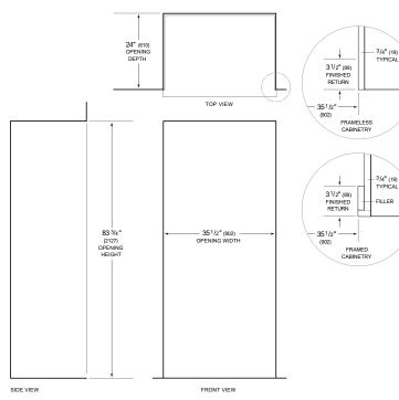
$NOTE: 3^{1}\!\ell^{a}$  (89) finished returns will be visible and should be finished to match cabinetry Shaded line represents profile of unit.
