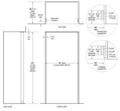
NOTE:  $3^{1}/2^{n}$  (89) finished returns and shaded areas will be visible and should be finished to match cabinetry. Shaded line represents profile of unit with  $3/4^{n}$  (19) panel.
