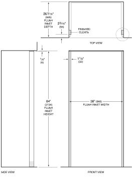
NOTE:  $3^{1/2^{\prime\prime}}$  (89) finished returns and shaded areas will be visible and should be finished to match cabinetry Shaded line represents profile of unit with  $3^{1/4^{\prime\prime}}$  (19) panel.
