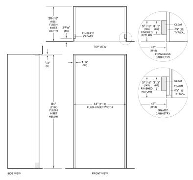
NOTE:  $3^{7}/2^{n}$  (89) finished returns and shaded areas will be visible and should be finished to match cabinetry. Shaded line represents profile of unit with  $3/4^{n}$  (19) panel.
