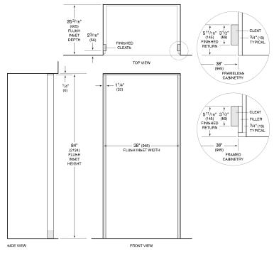
NOTE:  $3^1y_2^{\prime\prime}$  (89) finished returns and shaded areas will be visible and should be finished to match cabinetry. Shaded line represents profile of unit with  $3^1/4^{\prime\prime}$  (19) panel.
