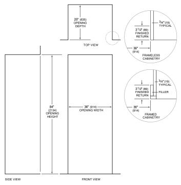
NOTE: 31/2" (89) finished returns will be visible and should be finished to match cabinetry
