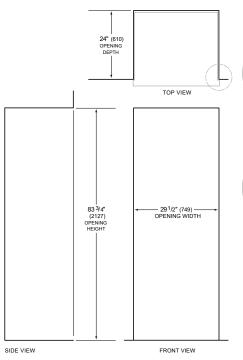
NOTE:  $3^{1/2^{\prime}}$  (89) finished returns will be visible and should be finished to match cabinetry Shaded line represents profile of unit.
