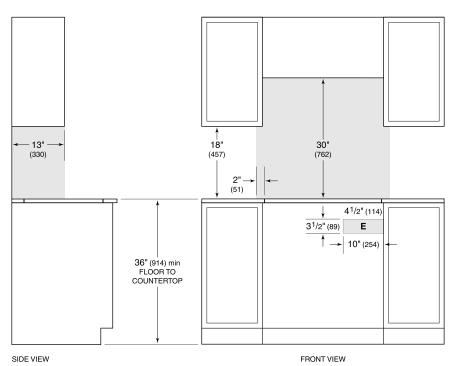
NOTE: Shaded area above countertop indicates minimum clearance to combustible surfaces, combustible materials cannot be located within this area. Electrical supply location only applies to installations with built-in oven.
