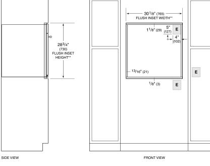
\*1" (25) minimum depth. Shaded areas will be visible and should be finished to match cabinetry. \*\*Dimension provides minimum reveals.
