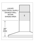
$\ensuremath{\text{NOTE:}}$  Dimensions in parenthesis are in millimeters unless otherwise specified
