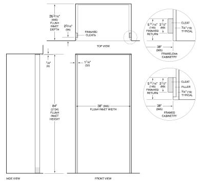
NOTE: 3<sup>1</sup>/2" (89) finished returns and shaded areas will be visible and should be finished to match cabinetry.
